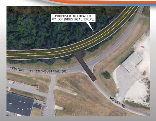
3. Reconstruct 2 curves from a 35mph design speed to a 45mph design speed.
